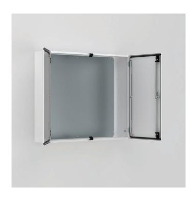
The mild steel double door wall mounted enclosure range, MAD, is ideal for installation in confined spaces where a single door, when opened, would take up too much space in front of the enclosure. The doors' loading capacity also increases as it is divided over two doors. With a IP 55 protection degree, components inside the enclosure are well protected and makes it well suited for many different applications.
